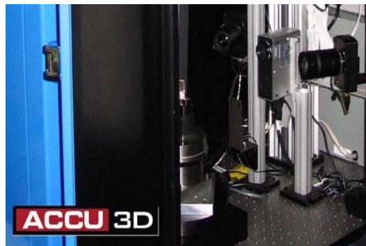
Cooling air hole inspection
