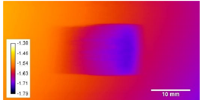
Figure 2: Top view of the surface of the same sample as Figure 1 (color represents depth)
