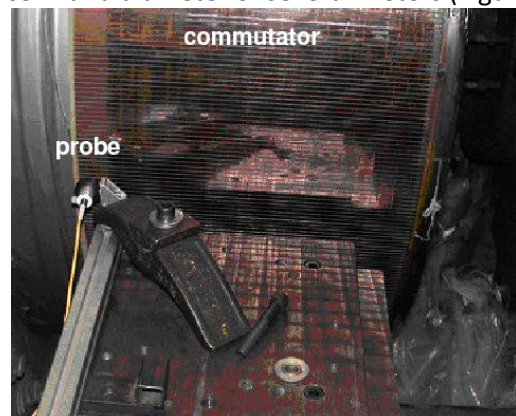
Figure 3: The probe of a fiber-based profilometer can scan large objects such as commutators
